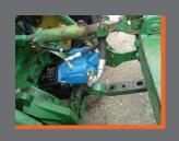
Our pressure compensating pumps used on all HydraBoost units allow for seamless changes in flow requirements. The flow self-adjusts to match itermittent usage items, such as compressors, without interruption of other hydraulic functions.
