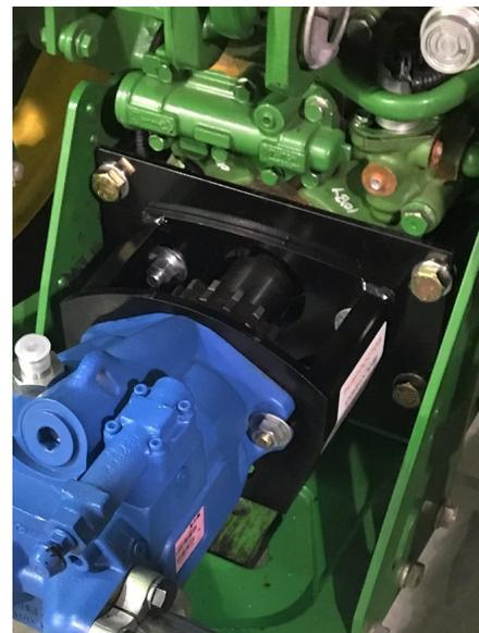
PumpDoctor attached to PTO pump
